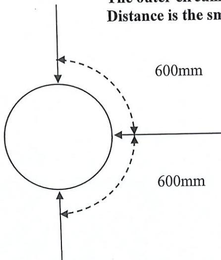
4) Thermocouple can be placed as per the client's requirement or at a regular interval of 0.5m on plate type joints.
