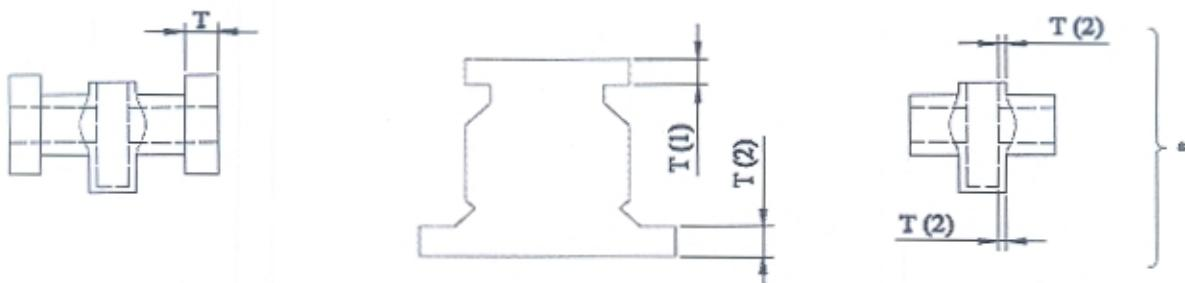
When all internal and external surfaces during heat treatment are within 13mm (1/2 in) of the final surfaces,  $ER = 1\frac{1}{4}T$ . When all internal and external surfaces during heat treatment are not within 13mm (1/2 in) of the final surface, then  $ER = 2T$  on multi flanged components, T shall be the thickness of the thickest flange.
