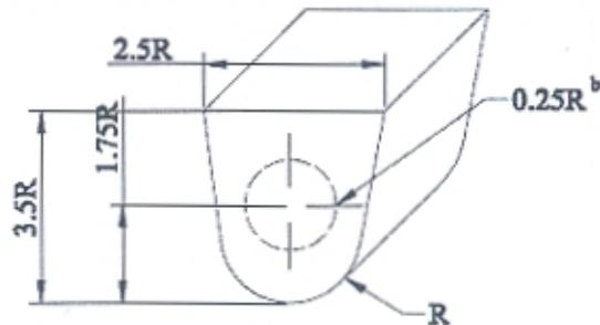
b. ENVELOPE FOR TEST SPECIMEN REMOVAL
