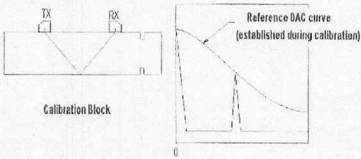
**CONDITION A - CALIBRATION BLOCK**
